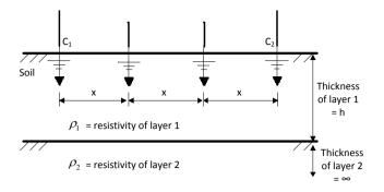
Figure 3: Two layer resistivity soil profile
