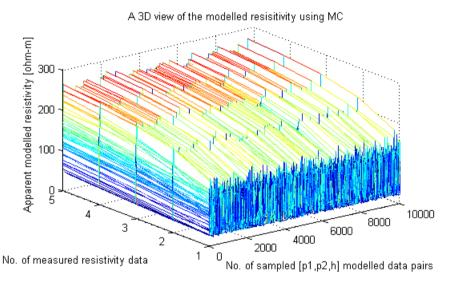
Figure 11: A mesh plot of all the modelled apparent soil resistivity solution set for case 4 data
