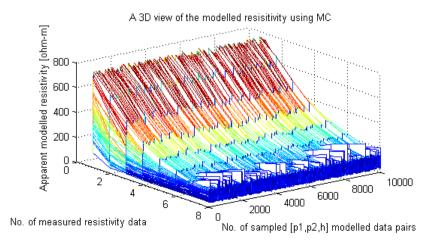
Figure 9: A mesh plot of all the modelled apparent soil resistivity solution set for case 3 data
