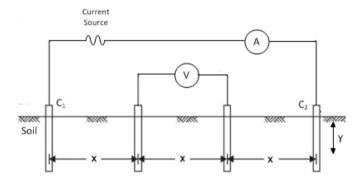
Figure 2: Wenner method measurement configuration
