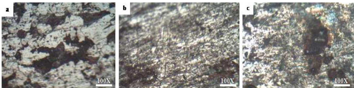
Figure 5: Microstructure of As - received a) 0.22 %C steel b) 0.24 %C steel c) 0.36 %C steel
