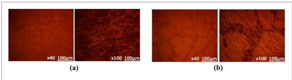
Figure 7. Microscopic images of (a) 3004Al and (b) 4044Al before corrosion test.
