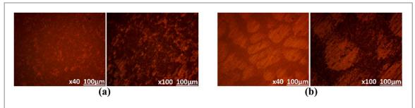
**Figure 11.** Microscopic images of (a) 3004Al and (b) 4044Al from 0.1 M H<sub>2</sub>SO<sub>4</sub> solution.
