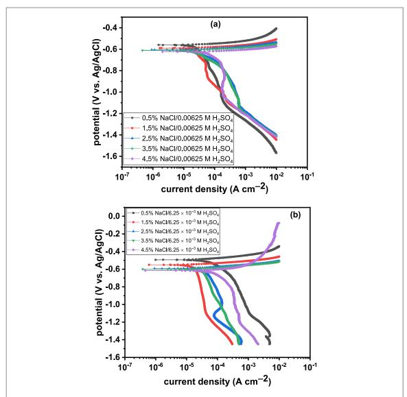
$\label{eq:figure 3. Potentiodynamic polarization plots of (a) 3004 Al alloy and (b) 4044 Al alloy in 0.00625 \ M\ H_2SO_4 solution in combination with 0.5\%-4.5\% \ NaCl solution at 30 °C.$
