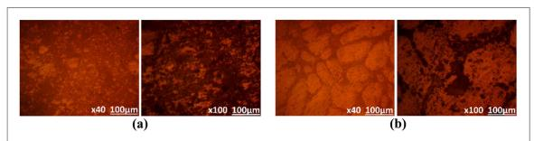
Figure 12. Microscopic images of (a) 3004Al and (b) 4044Al from 0.00625 M 0.1 M H<sub>2</sub>SO<sub>4</sub> solution at 0.5% NaCl concentration.
