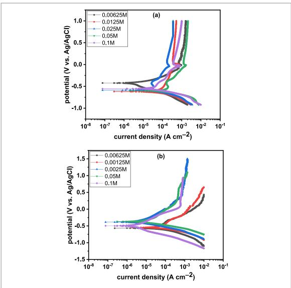
Figure 2. Potentiodynamic polarization plots of (a) 3004Al alloy and (b) 4044 Al alloy in different concentrations of  $\rm H_2SO_4$  solution at 30 °C.
