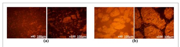
$\textbf{Figure 13.} \ Microscopic \ images \ of (a) \ 3004 Al \ and \ (b) \ 4044 Al \ from \ 0.1 \ M \ H_2 SO_4 \ solution \ at \ 0.5\% \ NaCl \ concentration.$
