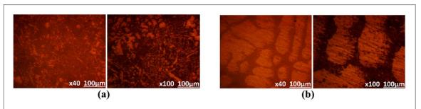
Figure 8. Microscopic images of (a) 3004Al and (b) 4044Al from 0.5% NaCl solution.
