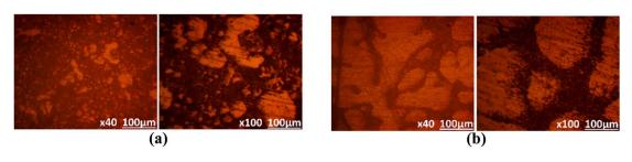
Figure 9. Microscopic images of (a) 3004Al and (b) 4044Al from 4.5% NaCl solution.
