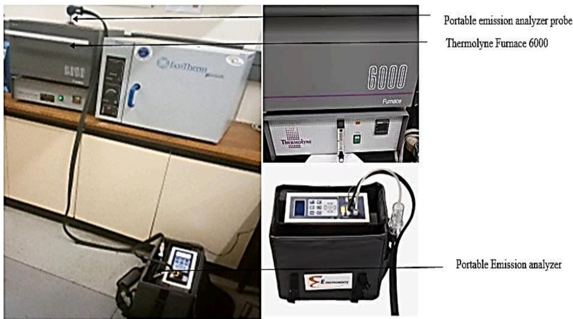
Fig. 5. Portable emission analyser and 950 °C thermolyne 6000 Oven.
