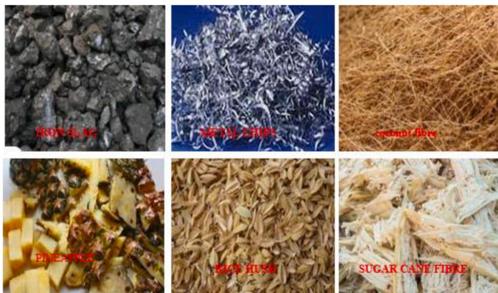
Fig. 2. Thermal insulators agro-industrial waste.
