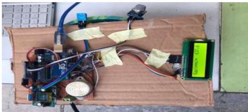
Figure 6: Picture of constructed device showing Carbon dioxide readings.
