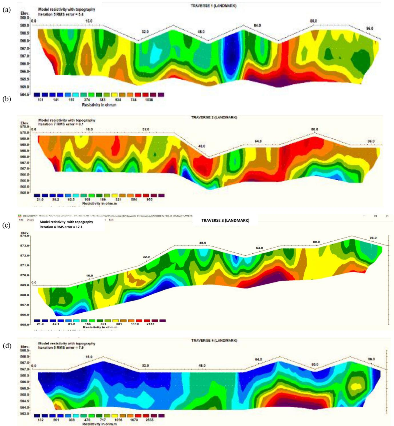
Figure 6. 2D resistivity inverse model for: (a) Traverse 1, (b) Traverse 2, (c) Traverse 3; and (d) Traverse 4 at Landmark University farm.
