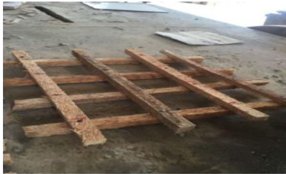
Fig. 2. Coconut palm stem strip reinforcement.
