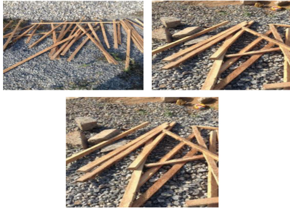
Fig. 1. (1-a) Coconut stem strips of size 16 mm x 15 mm. (1-b) Coconut strips of size 20 mm x 15 mm. (1-c) Coconut strips of size 25 mm x 15 mm.
