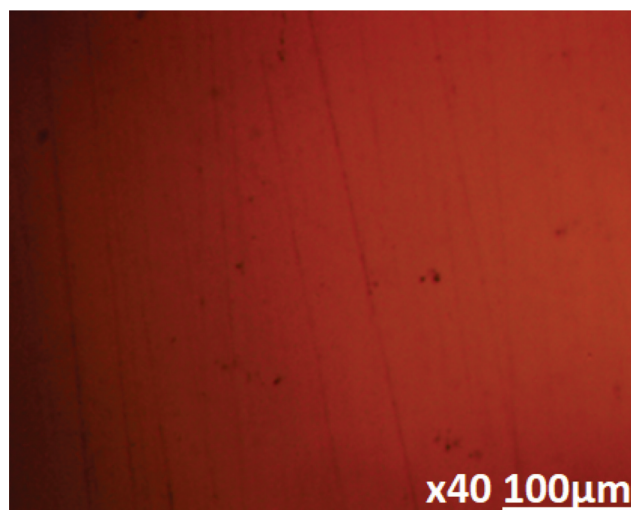
Figure 5. Optical illustration of 434FS prior to corrosion test.
