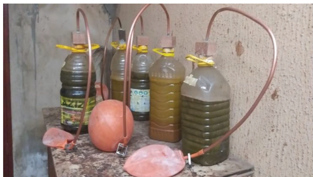
Figure 2. Laboratory set-up of common biogas collection from human waste.
