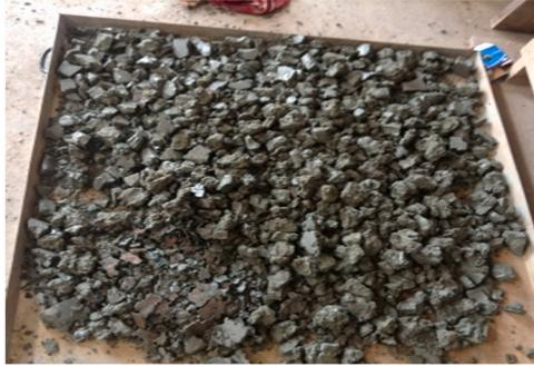
Fig. 3. Crushed plastic after melting.
