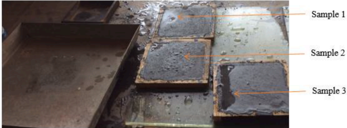
Fig 3. Developed ceiling composite samples.
