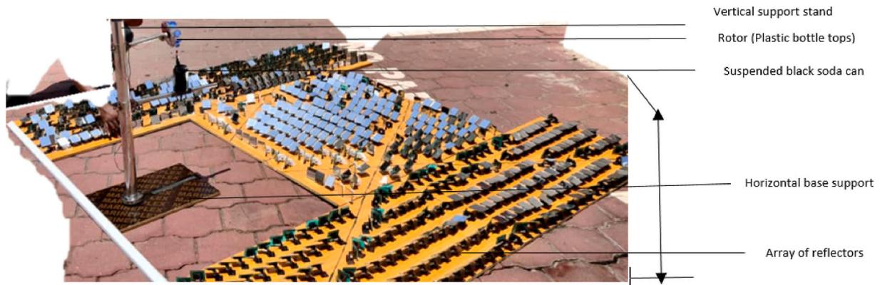
Fig. 1. Cross-section of STEG set-up.
