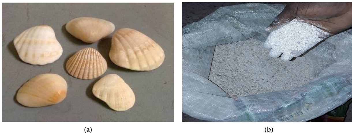
Figure 2. Senilia senilis seashells. (a) Before crushing; (b) after crushing.
