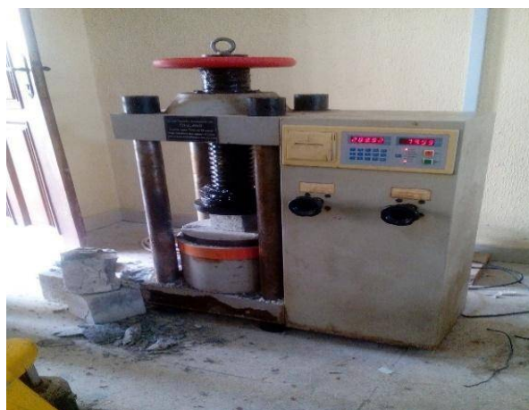
Figure 4. Compression testing machine for compressive and splitting tensile strength tests.
