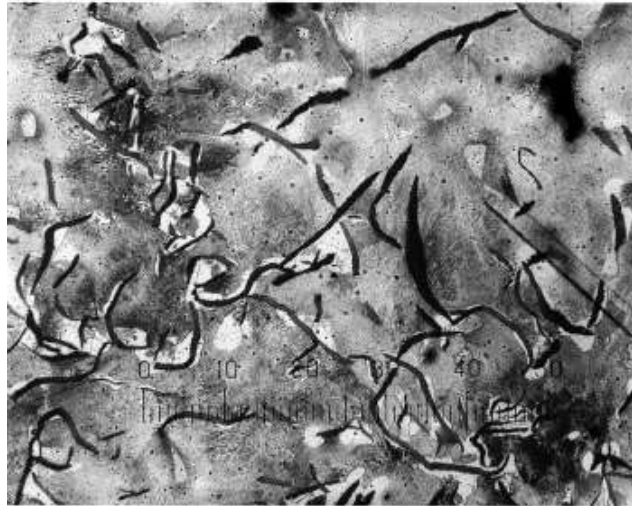
Fig 17: Micrograph of grey cast iron showing graphite flakes in a ferritic matrix
