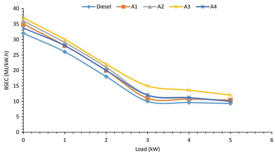
Fig. 10. Variation of Brake Specific Energy Consumption (BSEC) with Load.
