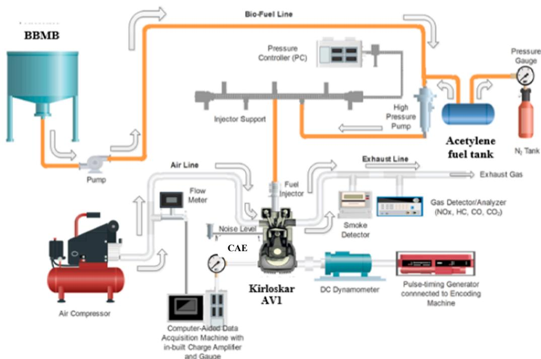
Fig. 2b. Engine test equipment for Kirloskar AV1 which shows the most important elements.
