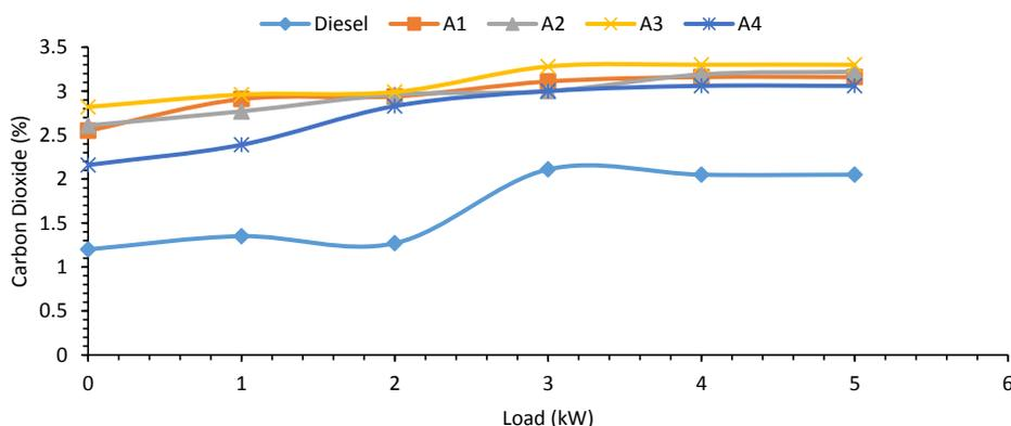
Fig. 15. Variation of CO<sub>2</sub> with Load.
