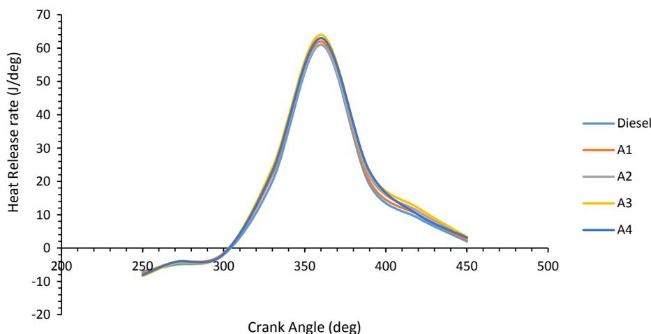
Fig. 5. Variation of Heat Release Rate with Crank Angle at Constant Load.
