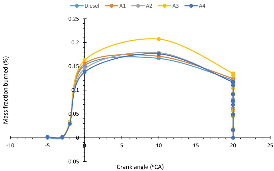
Fig. 14. Variation of mass fraction burned with crank angle.
