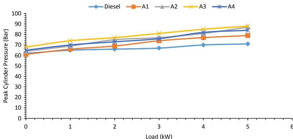
Fig. 6. Variation of Peak Cylinder Pressure with Load.
