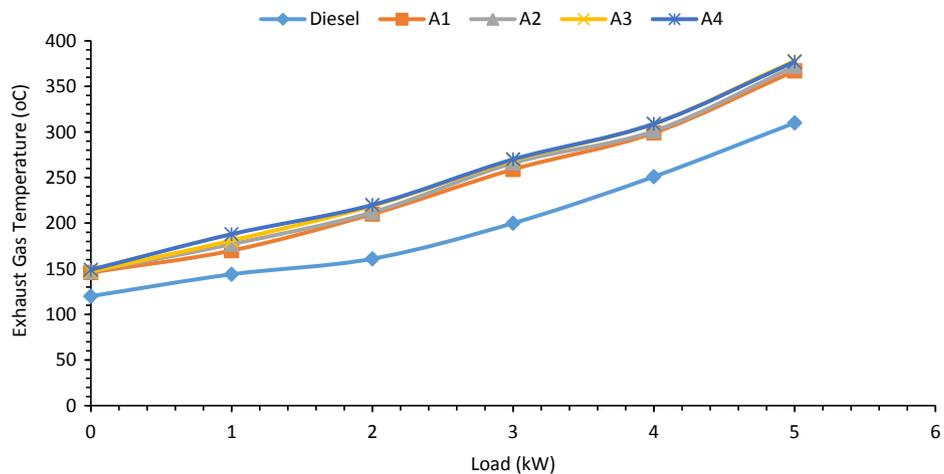
Fig 9. Exhaust Gas Temperature with Load.
