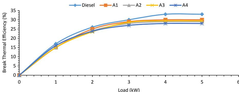
Fig. 8. Variation Brake Thermal Efficiency (BTE) with Load.
