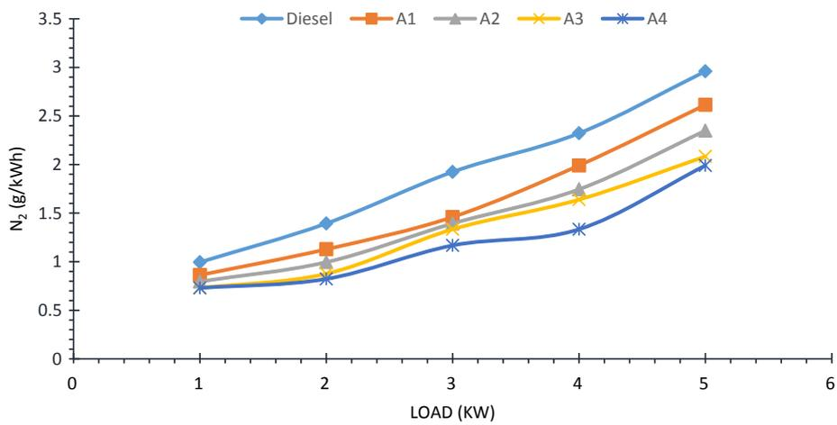
Fig. 13. Variation of NOx with Load.
