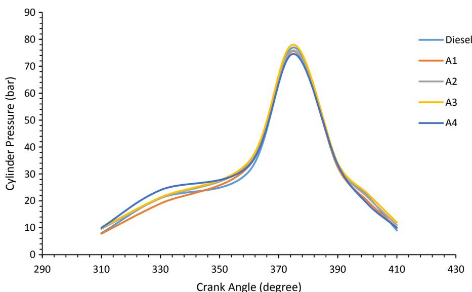
Fig. 4. Cylinder Pressure with Crank Angle at Constant Load.
