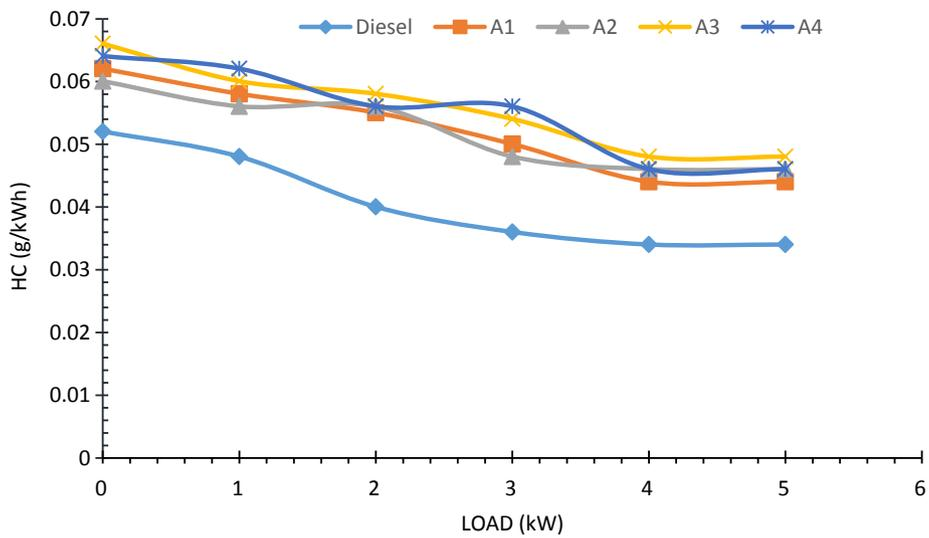
Fig. 12. Variation of Unburnt Hydrocarbons with Load.
