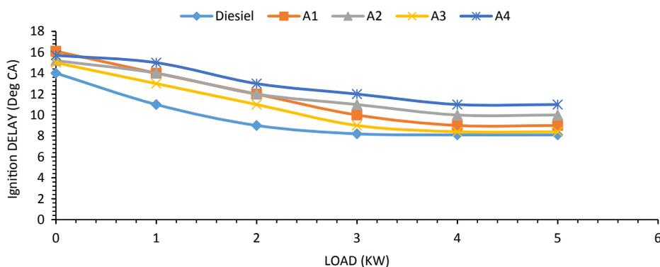
Fig. 7. Variation of Ignition Delay with load.
