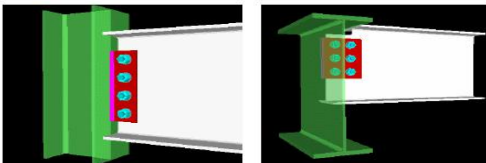
Figure 3. Typical Fin Plate Connection (a) Beam to Column (b) Beam to Beam [8].
