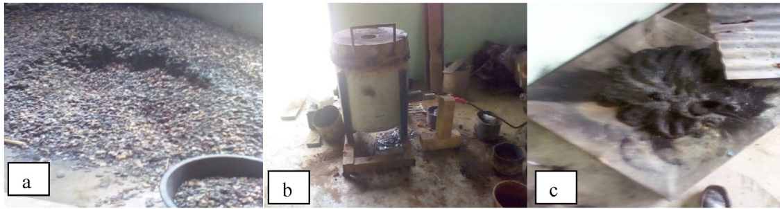
Fig. 1. (a) Cashew nutshell (CNS) (b) burning of CNS in a gas furnace and (c) CNSA.
