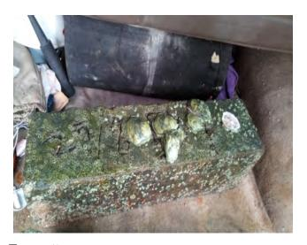
Figure 5: Beam buried in Lagoon water after 1 year.
