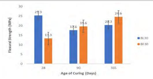
Figure 4: Flexural strength result
