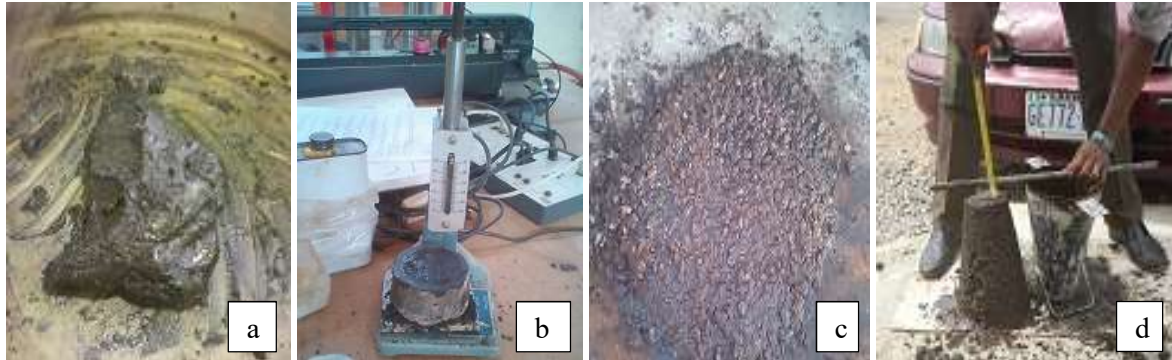
Figure 1. The workability tests (a) paste (b) setting time (c) fresh concrete mix (d) slump
