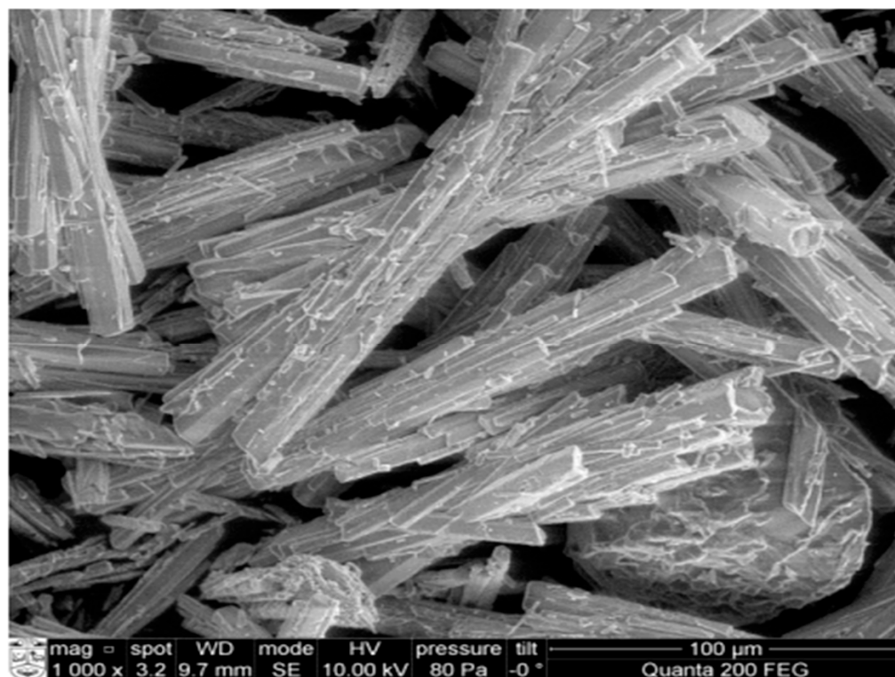
Figure 7. Morphology of phosphogypsum [98].
