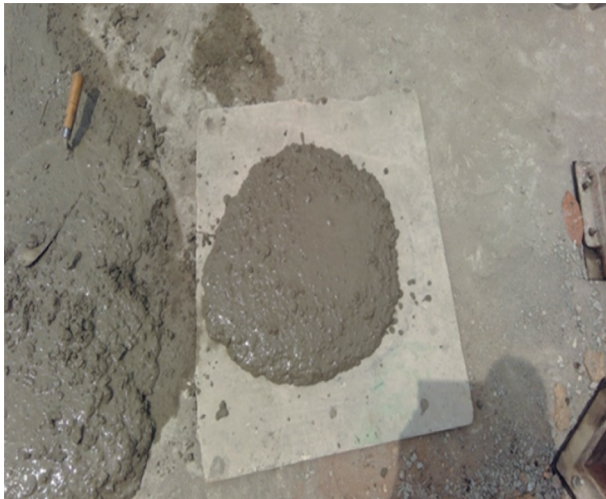
Figure 3. Slump Flow T 50 .
