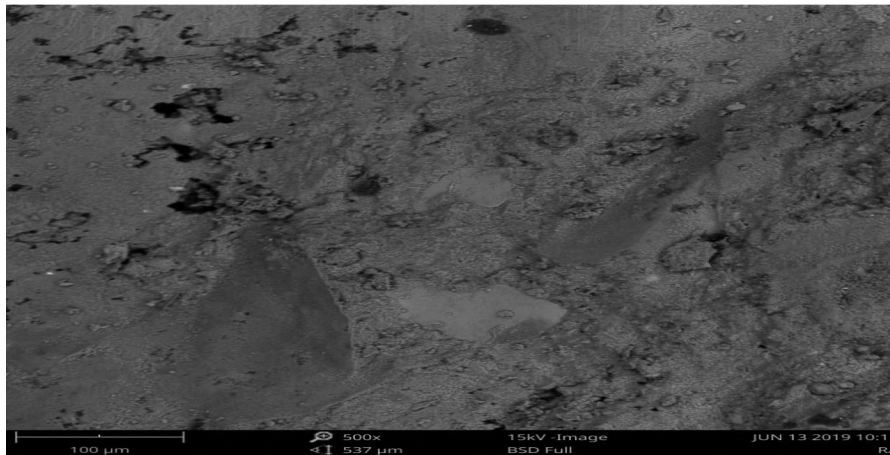
. SEM Micrograph of recycled aggregate at 10% replacement
