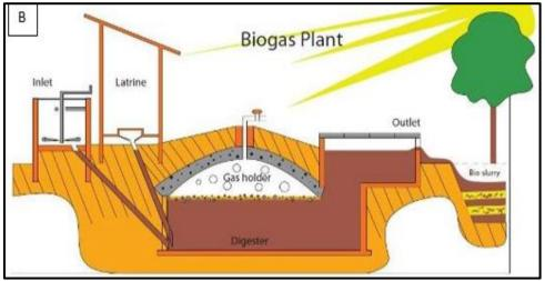
(b) The Biogas production process [1]
