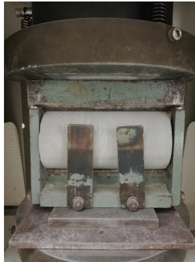
Fig. 5. Setup for splitting tensile test
