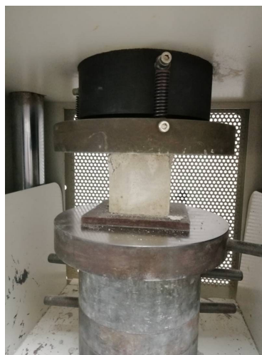
Fig. 4. Apparatus for compression testing
