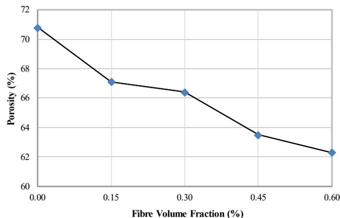
**Fig. 6.** Porosity of LFC with various MAF volume fractions
