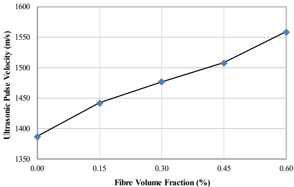
**Fig. 8.** Ultrasonic Pulse Velocity of 550kg/m<sup>3</sup> LFC with various MAF volume fractions
