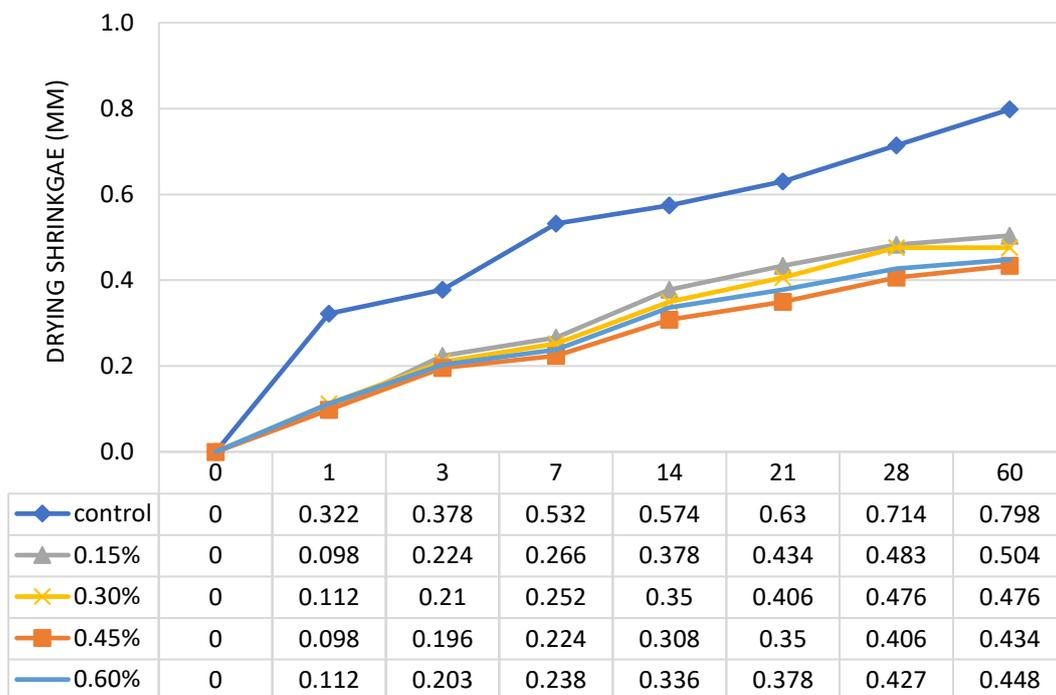
Fig. 7. Drying shrinkage of 550kg/m<sup>3</sup> density with various MAF volume fractions
