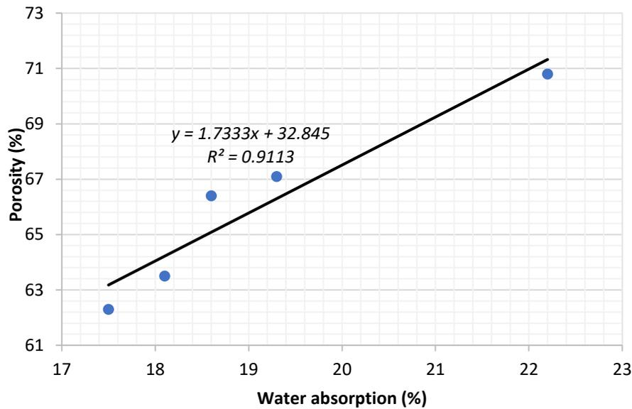
Fig. 9. Relationship between water absorption and porosity
