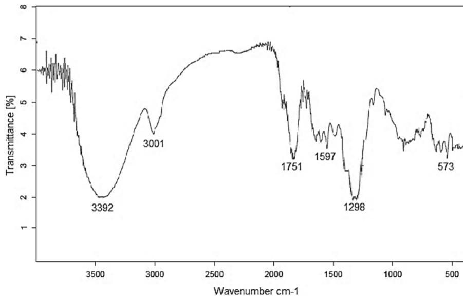
**Fig. 2.** FTIR spectrum for MAF
