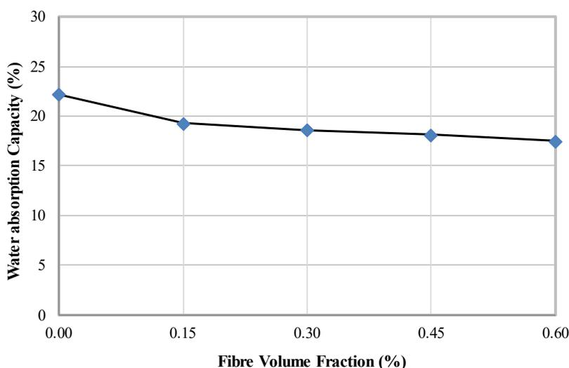
**Fig. 3.** Water absorption of  $550 \text{ kg/m}^3$  with various MAF volume fractions
