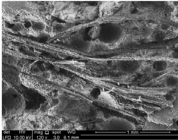
**Fig. 5.** Morphology of LFC with the inclusion of 0.3% of MAF
