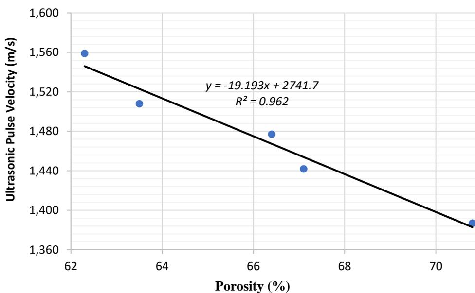
Fig. 10. Relationship between porosity and ultrasonic pulse velocity
