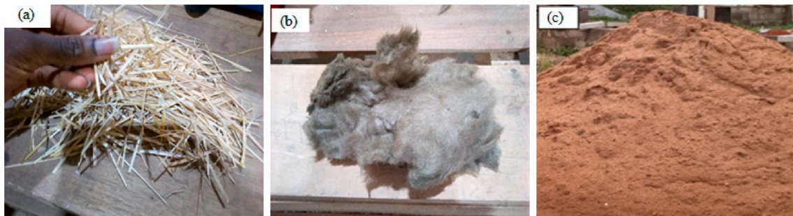
Fig. 1. Raw materials used for mortar production: (a) rice straw; (b) rock wool; and (c) river sand.
