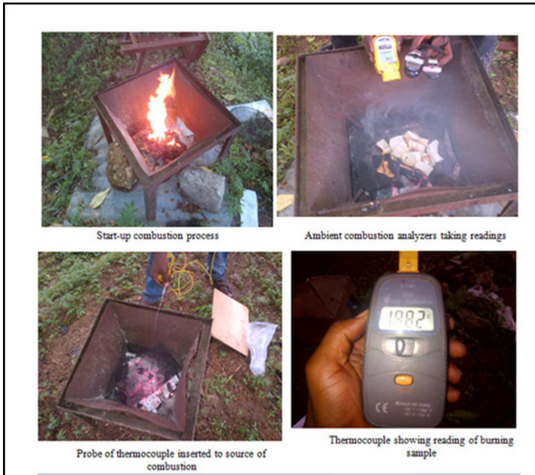
Fig. 2. The stages of the ceiling material combustion.
