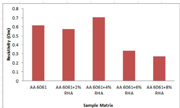
**Fig. 7.** Resistivity of RHA reinforced AA6061.
