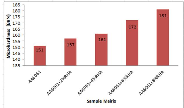
**Fig. 4.** Effect of RHA content on Microhardness.
