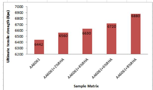
**Fig. 5.** Effect of RHA particles on Tensile Strength.
