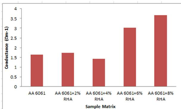
**Fig. 6.** Conductance of RHA reinforced AA6061.
