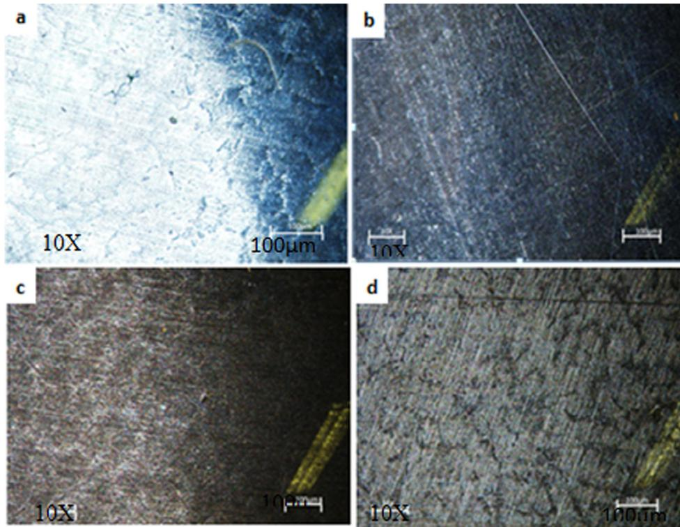
**Fig. 2.** (a): Optical micrograph for AA6061 + 2%RHA (b) Optical micrograph for AA 6061 + 4% RHA (c) Optical micrograph for AA 6061 + 6% RHA (d) Optical micrograph for AA 6061 + 8% RHA.
