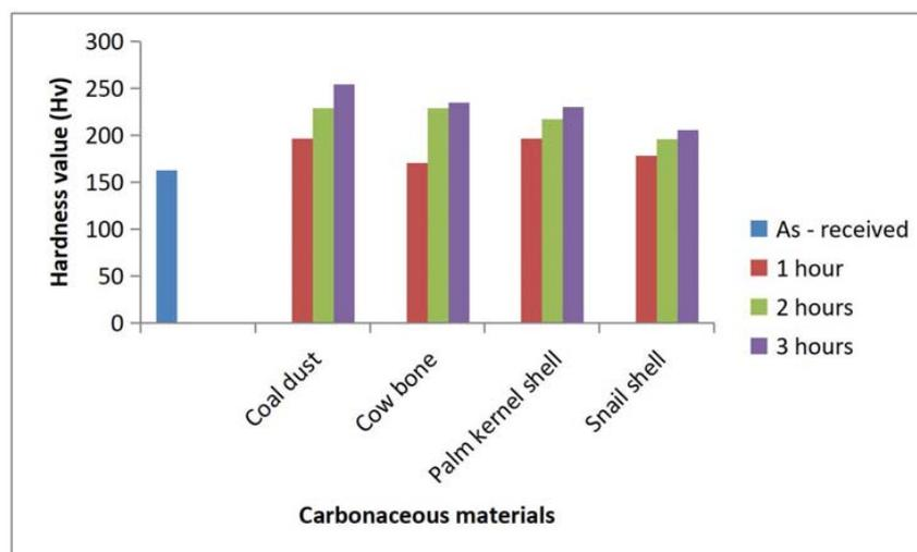
Figure 1: Effect of some carbon rich materials and varying soaking time on the hardness property of low alloy carbon steel
