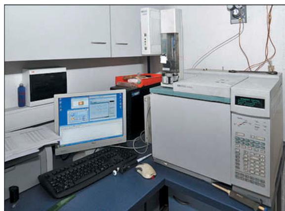
automatic injector system and oven cryocooling gives room for exact measurement of retention attributes of volatile compound for accurate estimation of their physical properties.
