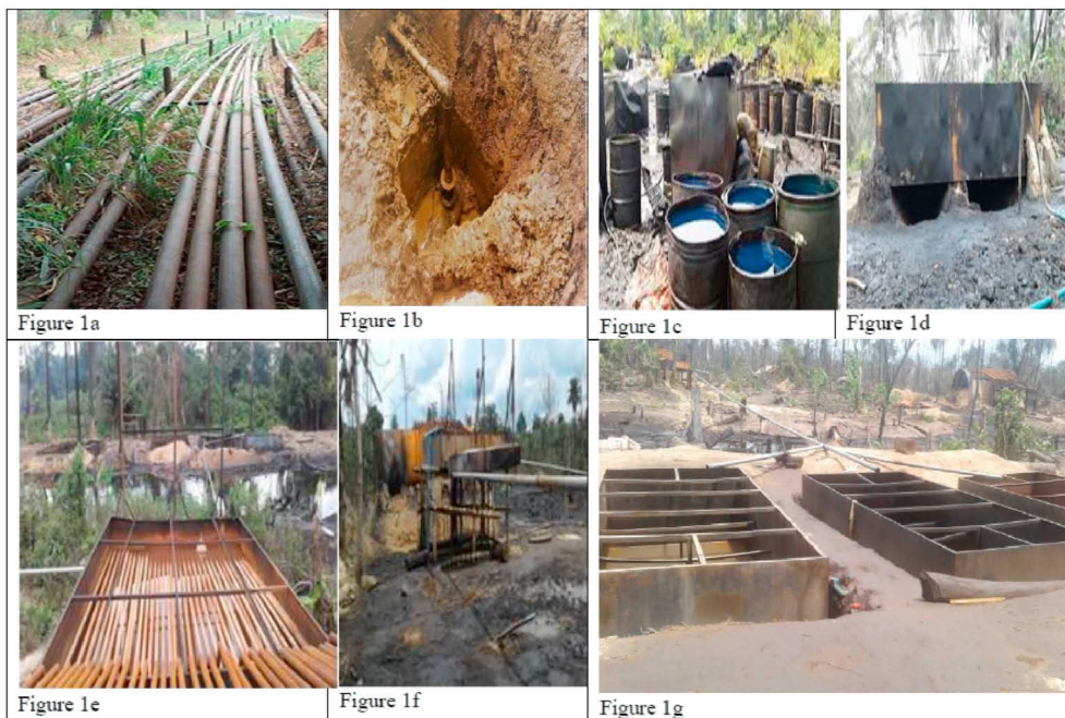
Figure 1. (a–g): Typical Artisanal Petroleum Refinery Flow Chart from Raw Material (crude oil) Acquisition to Refined Products Delivery.
