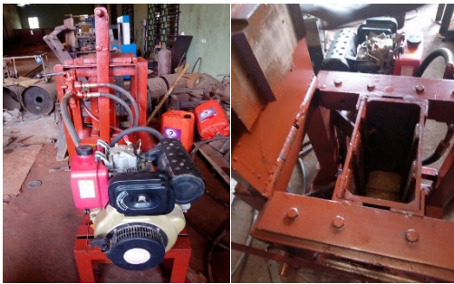
Fig. 1(c) NBRRI interlocking block machine used
