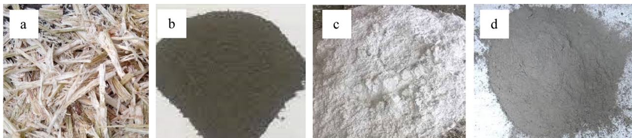
Fig. 1. (a) Sugar cane bagasse; (b) Sugar cane bagasse ash; (c) Calcite powder; (d) Portland limestone cement.
