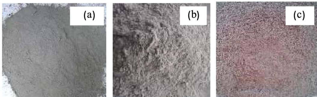
Fig. 1. Binding materials used (a) PLC (b) GGBFS (c) CCA.
