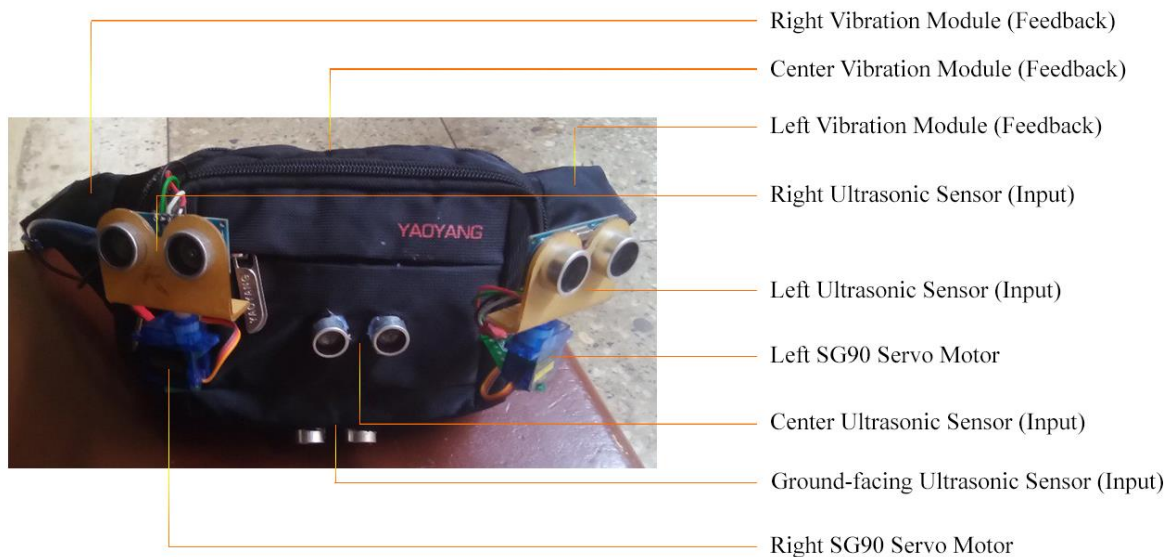
Figure 7 The Visuomotor Augmentative Sensory Aid (VASA)
