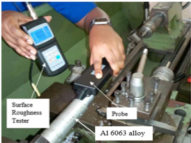
**Fig. 1** During the experiment, the cutting zone, and the surface roughness tester
