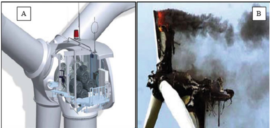
Fig. 11 a Design of the planetary gear in the nacelles compartment. b The failure of the wind turbine (WT) during operation
