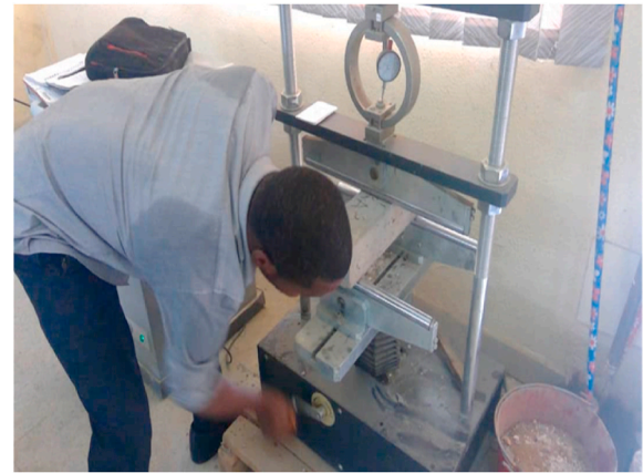
Fig. 2. Flexural test on beams.
