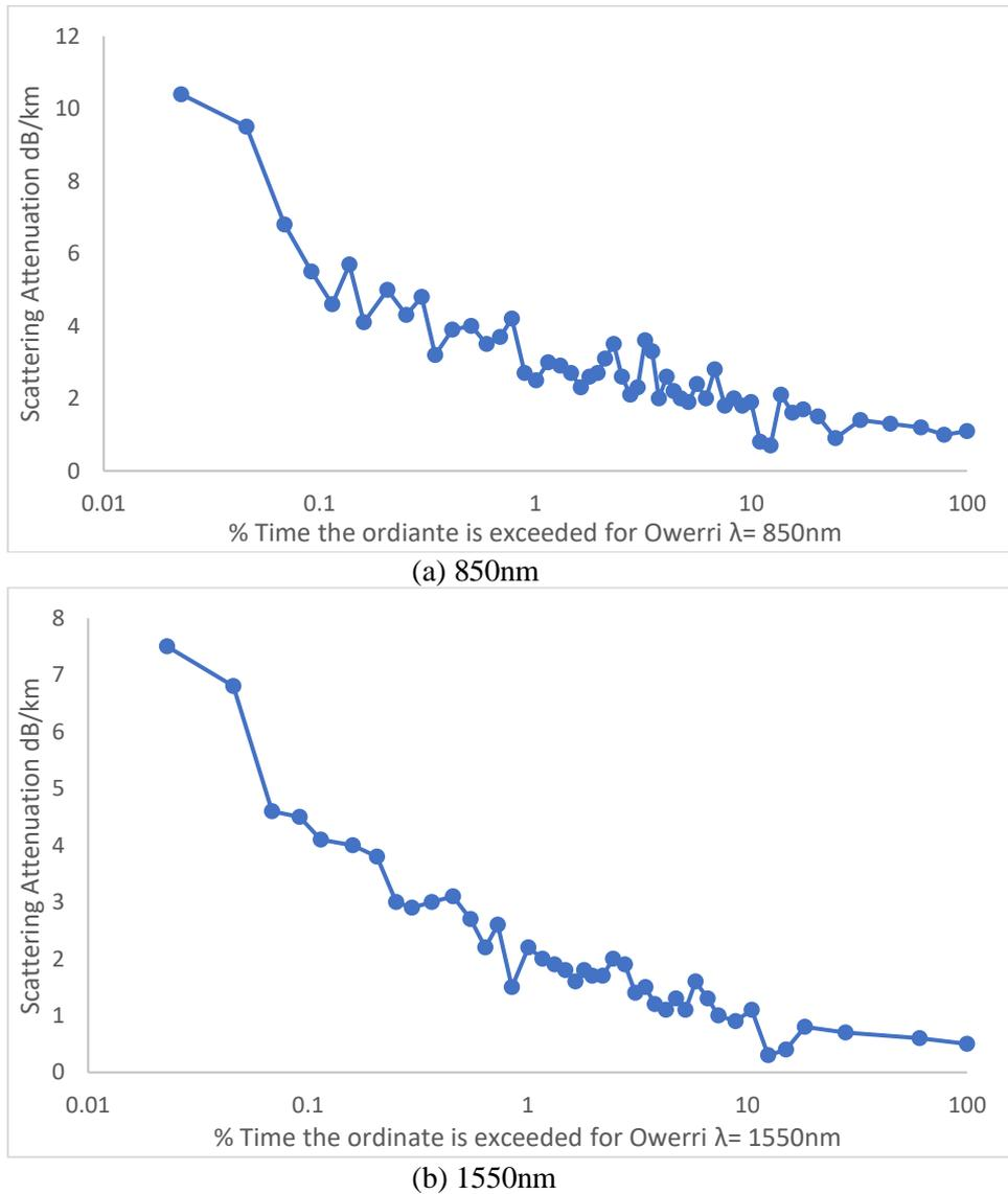
**Figure 4:** Cumulative distribution of attenuation at (a) 850 nm/352 THz and (b) 1550 nm/193 THz.
