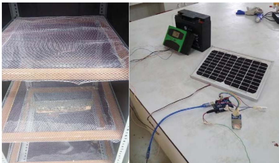
Figures 2.1 (a) and (b): Inside the Blackbody Solar Dryer and Connection of data logger powered with solar cell
