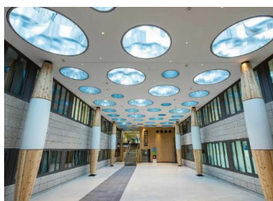
Figure 3: How light pipes light a space in a building (left)
