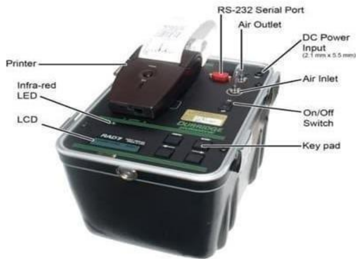
Figure 3: DurrIDGE Rad7 Radon monitor detector
