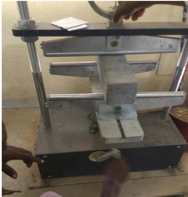
Fig. 2 Three-point bending test
