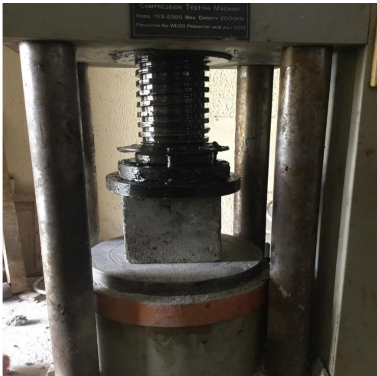
Fig. 1 Test sample in the compression testing machine
