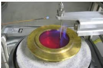
Fig. 6. Paint sample at fire point
