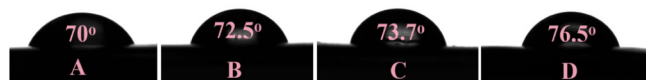
Fig. 7. Water contact angle of A= PU, B= 0.1% PU-GO, C= 0.3% PU-GO, D= 0.5% PU-GO.
