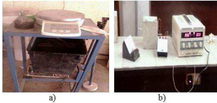
Fig. 3: Durability tests conducted on the hardened concrete: a) water absorption and total porosity tests, b) electrical resistivity test.
