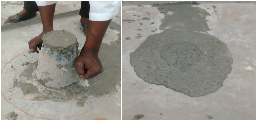
Fig. 4: Slump flow test.
