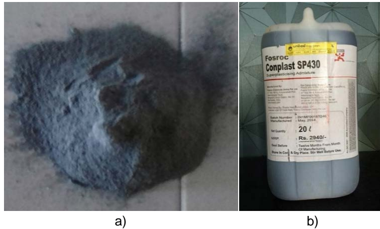
Fig. 2: Materials added to the concrete: a) induction furnace slag, b) Conplast SP 430 super plasticizer.
