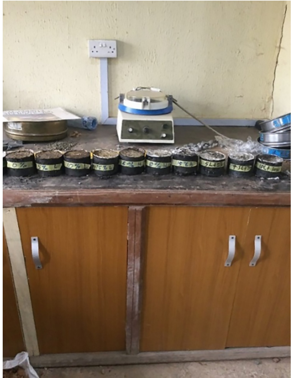
Fig 1. Test samples of the asphaltic RAP-HDPE-LDPE concrete.
