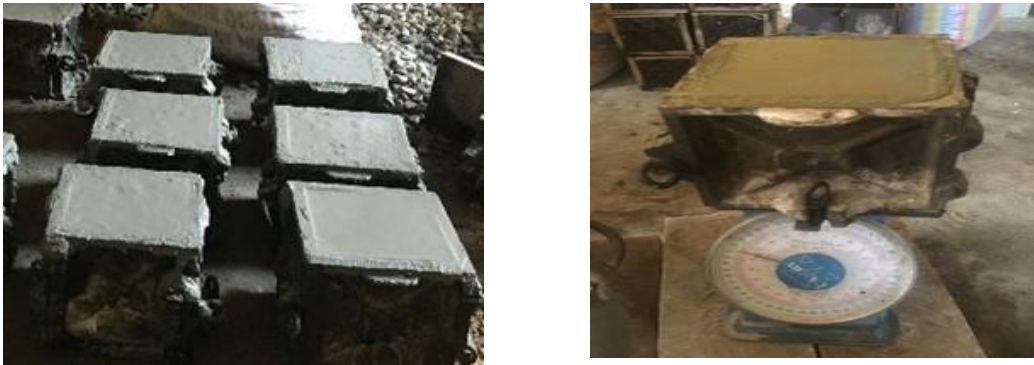
Figure 2. Freshly cast concrete cubes and wet density test
