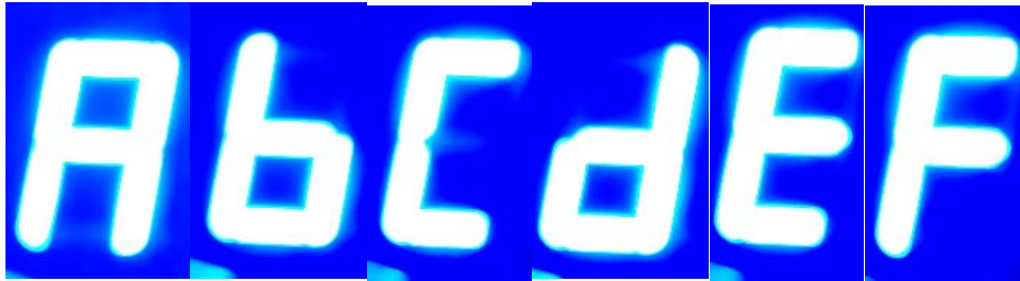
Figure 17: A blue 7 segment display displays number 0 – 9, A – F
