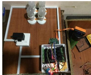
Figure 11. System testing with iron Figure 12. System testing to control load with four 60 W bulbs
