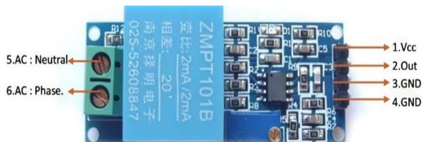
Figure 6. ZMPT101B voltage sensor
