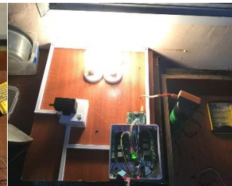
Figure 11. System testing with iron Figure 12. System testing to control load with four 60 W bulbs
